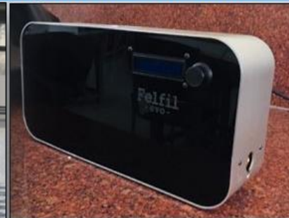
Single Screw Extruder (Felfil evo)
